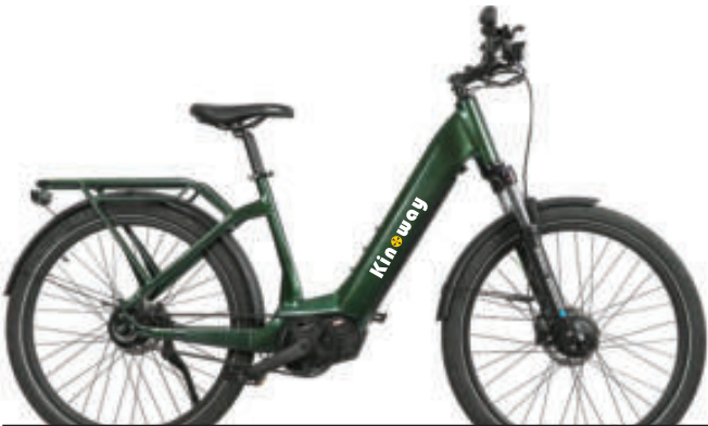
KV2708-1A Size:27.5" ● Gates-Belt Driving, LOFANDI Internal 3-Speed City eBike with ANANDA Mid-drive Motor
